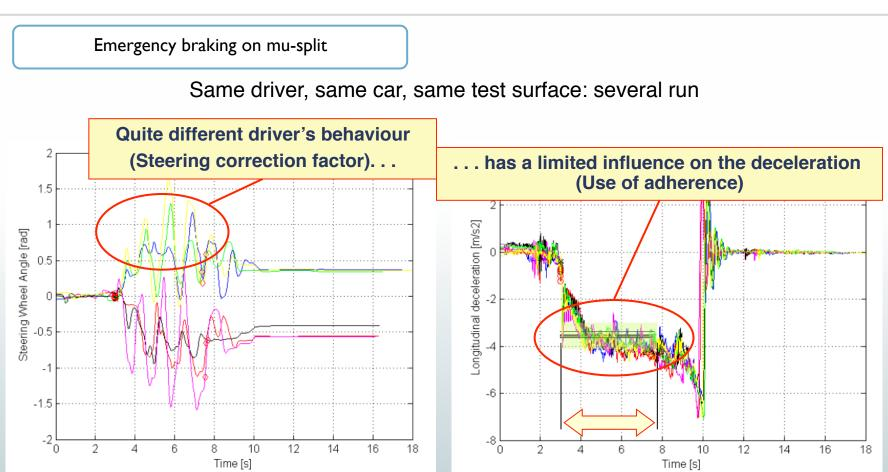
The steering wheel activity by itself does not look like a robust quantity to describe the vehicle behaviour, whereas the longitudinal deceleration looks quite stable despite the driver's actuation.
