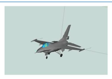
Neuro-muscular vibration amplified by the fly by wire (side stick) system causes the system to show unwanted roll-oscillation.
