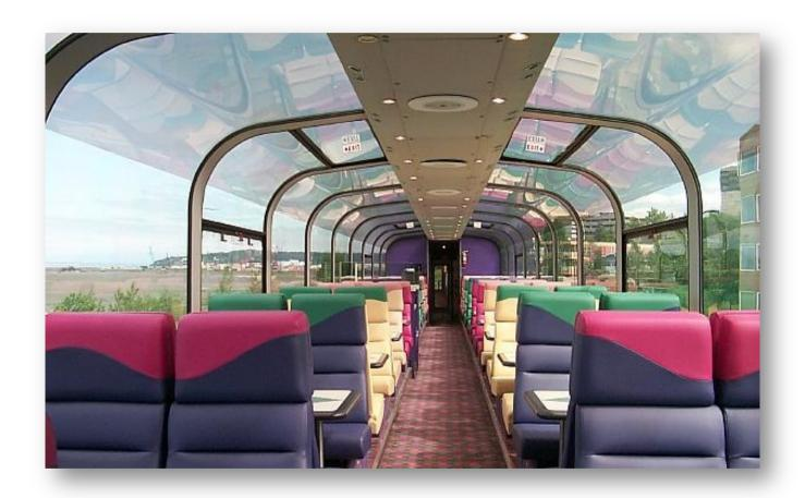
This is the interior of the single level "dome" car. A small galley is at the car end.
