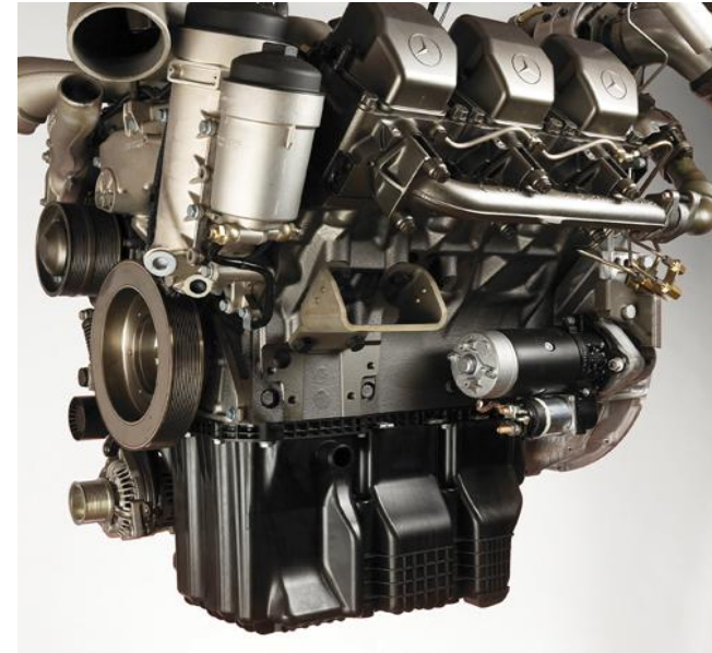
Daimler 2004 MY Actros BR500 Class B Ultramid A3HG7 Plastic Oil pan 50% Weight Reduction from Aluminum 1dB overall noise reduction
