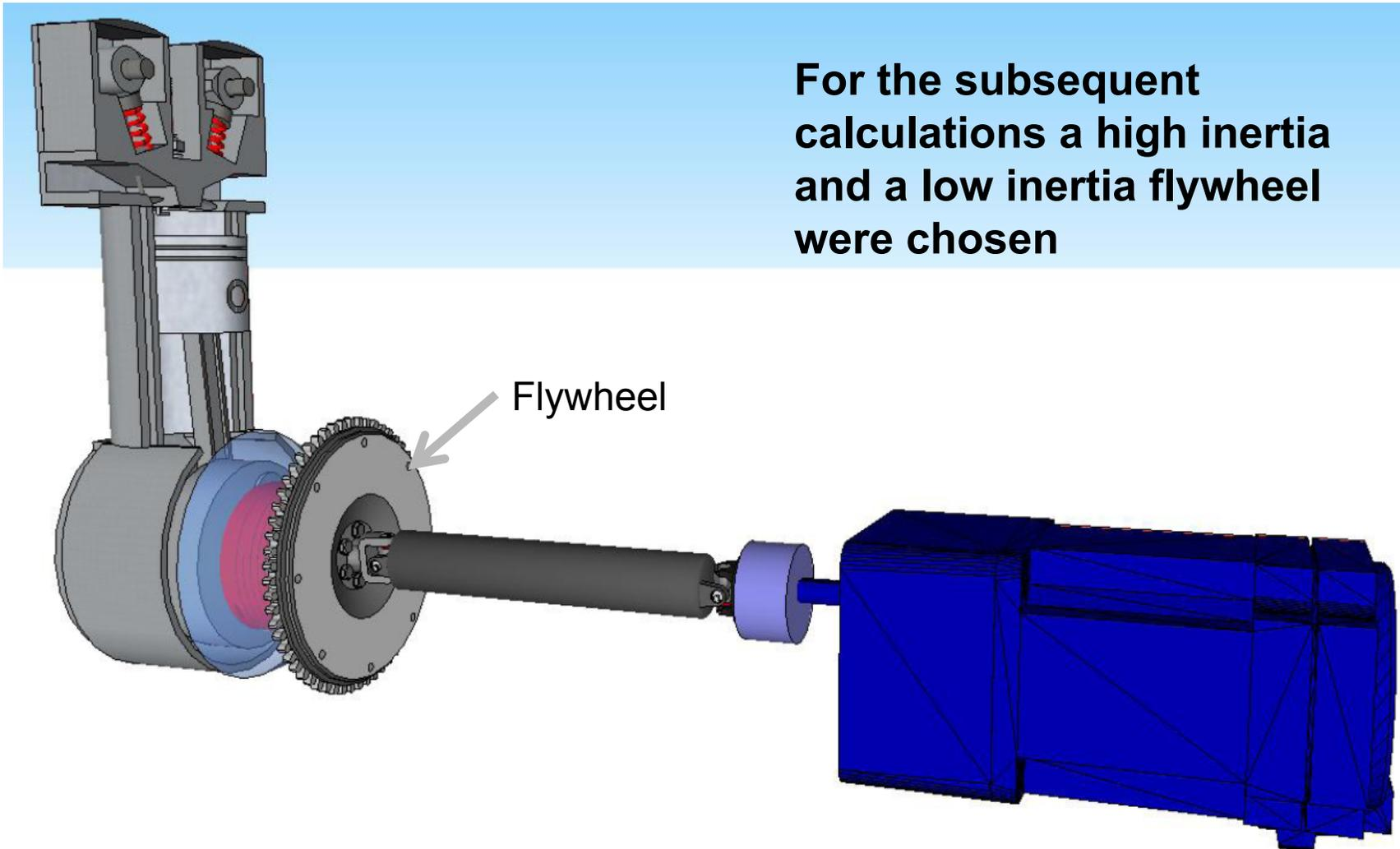
For the subsequent calculations a high inertia and a low inertia flywheel were chosen
