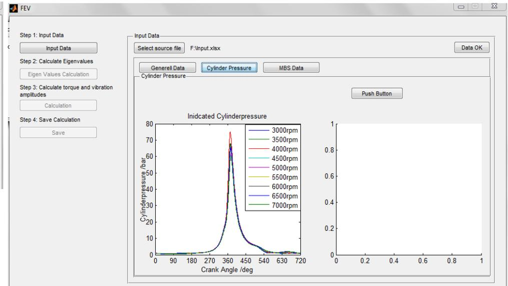
Cylinder pressure data (if pressure traces are not available, a function generator will create pressure traces using a provided peak cylinder peak)
