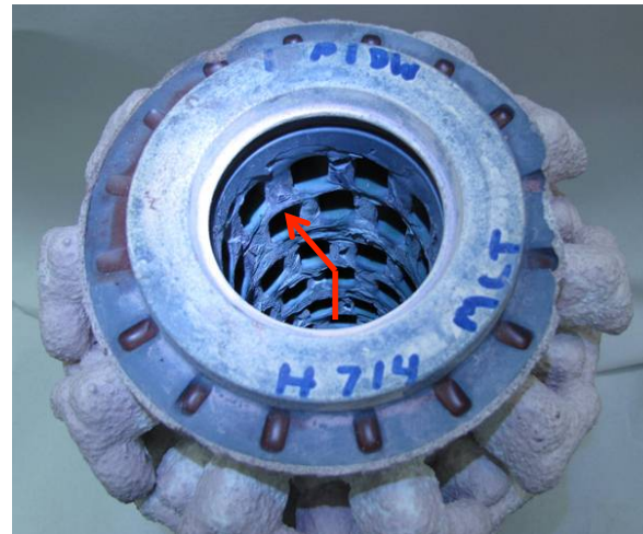
Ceramic Shell after dewax
